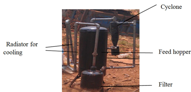
Figure 5. Experimental updraft gasifier.
